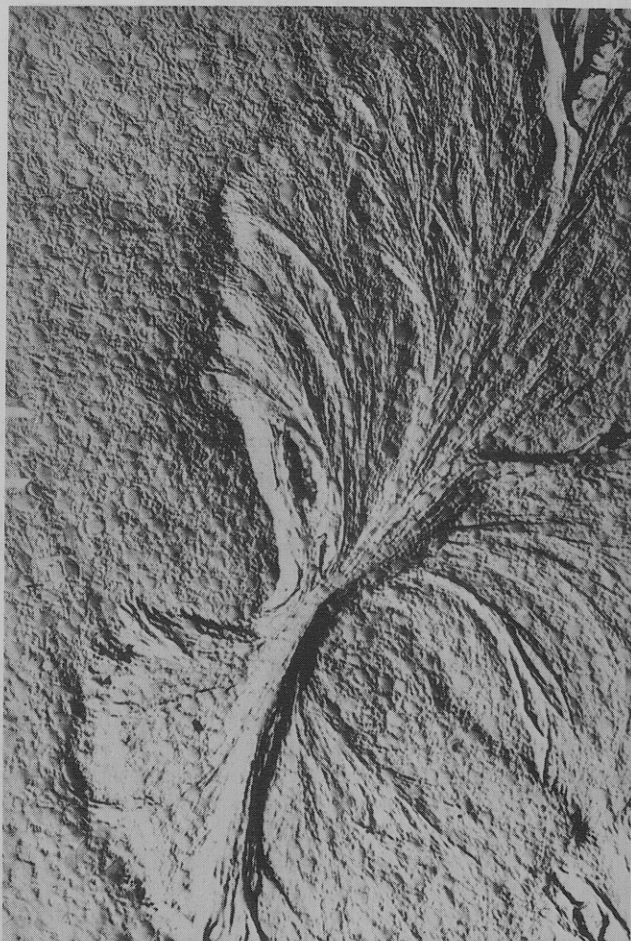
Figure 9. Replication electron micrograph of free surface of copolymer A cast from nitromethane. Reprinted with permission from ref 6. Copyright 1970 Plenum Press.
